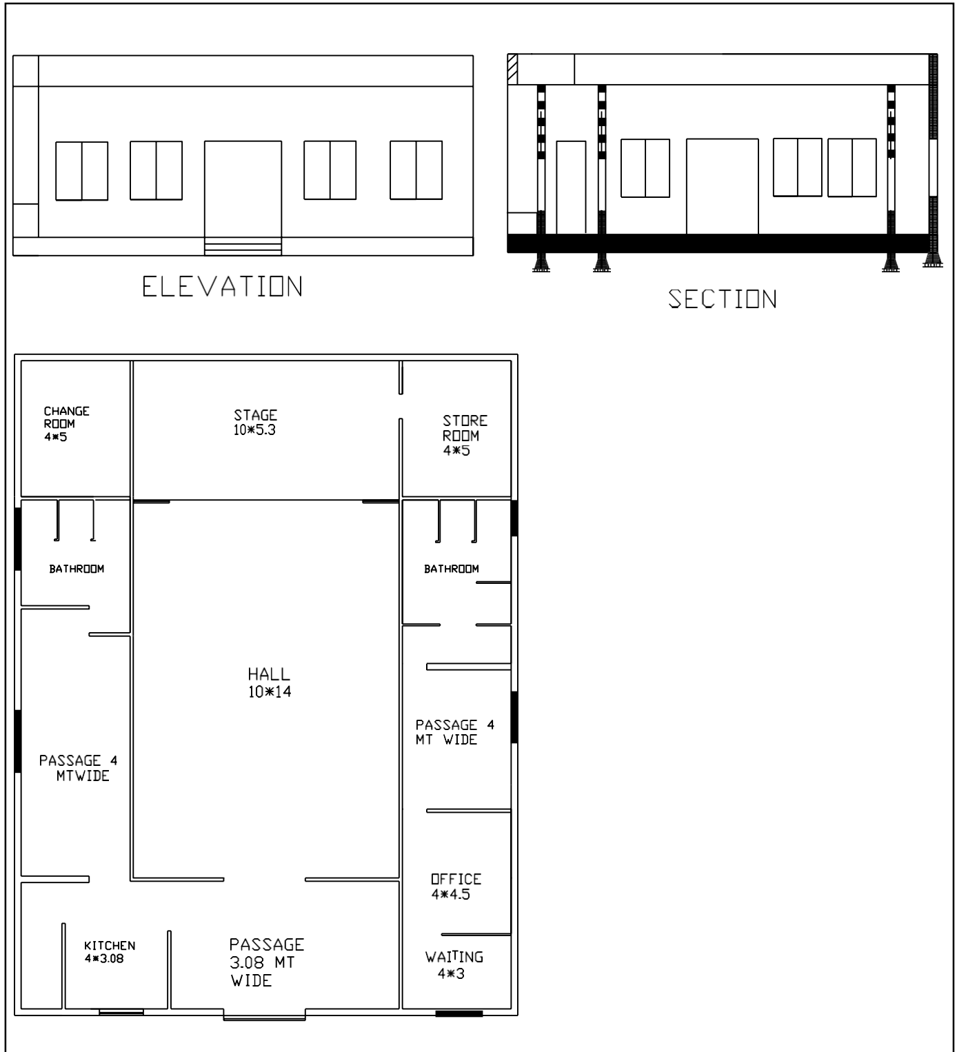
Figure 69 Plane, Elevation And Section Of Community Hall
